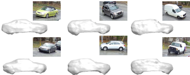
Figure 13. Vehicle Category Reconstruction. Our method is able to fuse videos of 365 vehicles with different appearance and shape into a category model. From left to right, we show reconstruction of sedans, SUVs, and vans.
