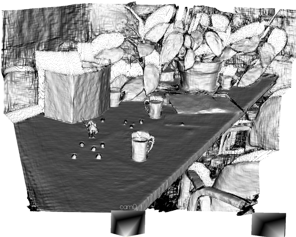
Figure 8: Reconstruction of HSM-F estimation on image Crusade-perfect by projecting disparity to world coordinates.
