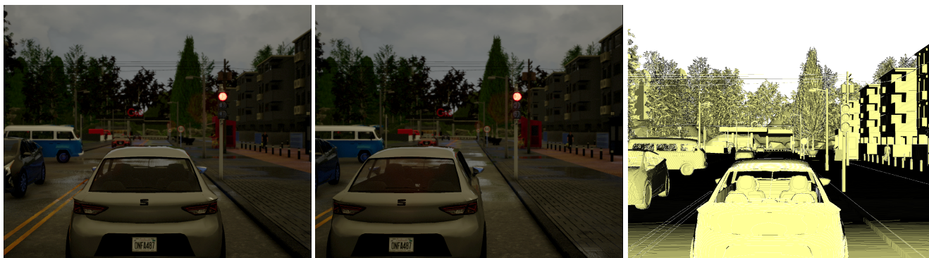
Figure 1: Example high-resolution rectified image pairs as well as projected ground-truth depth in HR-VS.
