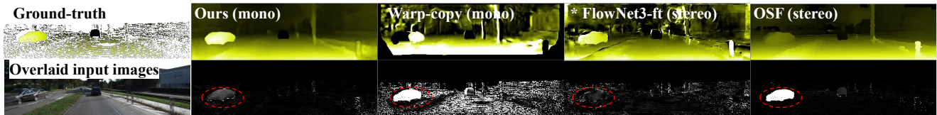
Figure 6. Results for image “000105” in the KITTI val set. Top: Motion-in-depth between two frames where bright indicates points moving towards the camera; bottom: error maps of motion-in-depth. Our method predicts more accurate motion-in-depth than the baselines.
