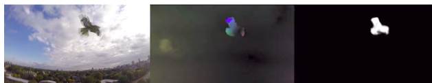
Figure 1. Optical flow vs optical expansion. From left to right: overlaid two consecutive frames, color-coded optical flow fields and optical expansion map, where white indicates larger expansion or motion towards the camera. Notice it is difficult to directly read the 3D motion of the hawk from optical flow. However, it is easy to tell the hawk is approaching the camera from optical expansion.
